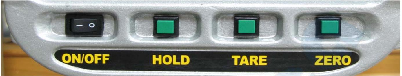
**ON/OFF key:** Turn the scale on/off, all segment and indicator LED are illuminated for one second, during display test, all internal operation are checked and, any non-conformance Error message will be displayed.
